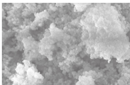
FIGURE 25 : SEM images from the NANOBADGE filters (source) showing highly agglomerated TiO 2 nanoparticles.
